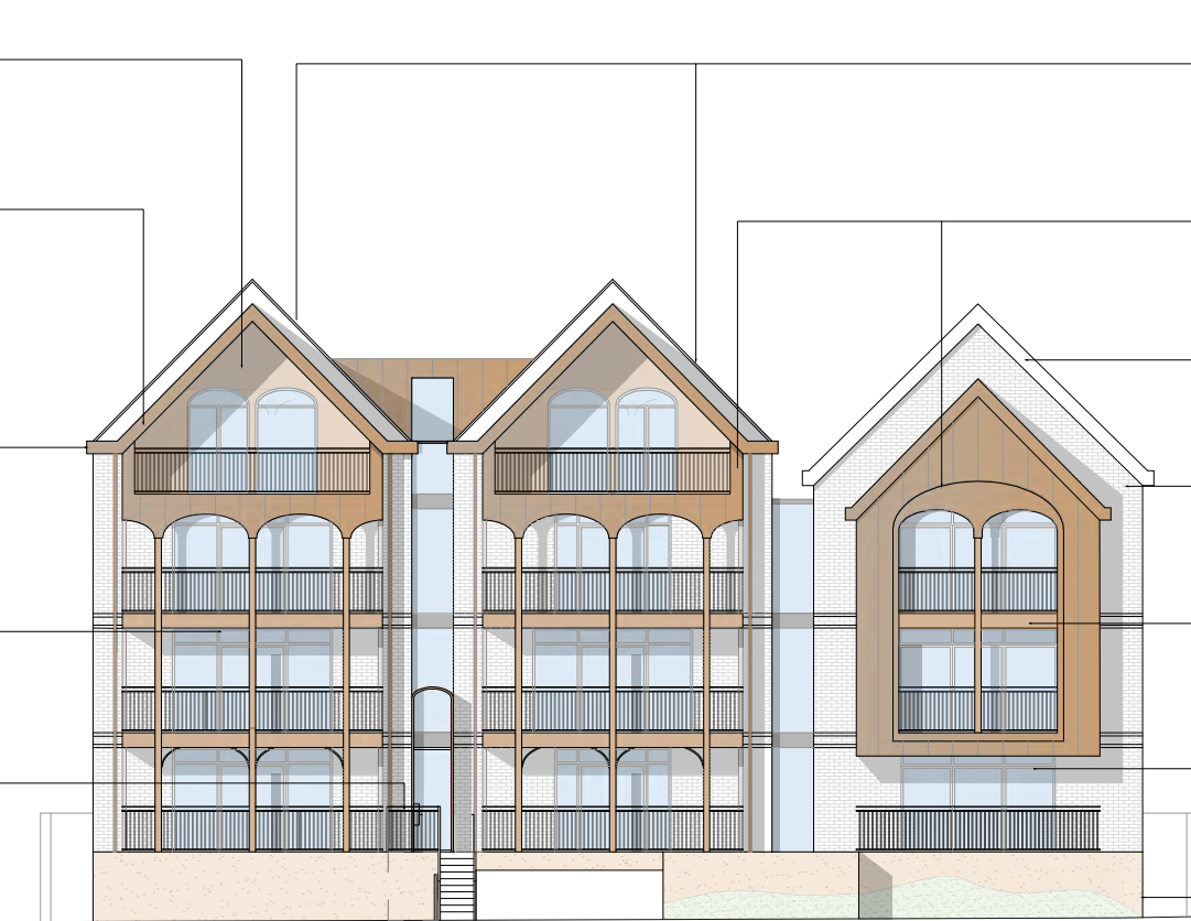
PROPOSED FRONT ELEVATION - MATERIALS 1:200 @ A3
